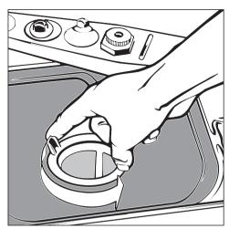
To unscrew the micro-fine filter, take hold of the two lugs, turn twice in an anti-clockwise direction.
